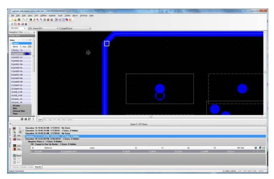
**Negative Plane - Drill spacing** checks include Through Hole Drill to Copper, Via Drill to Copper, Laser Via Drill to Copper, Updated Through Hole Drill to Copper, and Back Drill to Copper.
