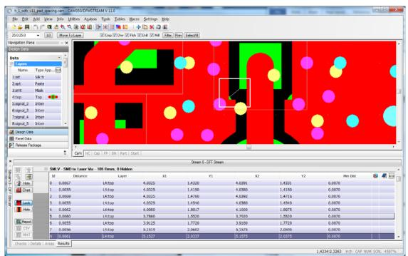
**Signal Layer - Drill spacing** checks include Unplated Through Hole Drill to Copper, Unplated Through Hole Drill to Pad, Unplated Through Hole Drill to Track, Back Drill to Copper, Back Drill to Pad, Back Drill to Track, Through Hole Drill to Copper, Through Hole Drill to Pad, Through Hole Drill to Track, Via Drill to Copper, Via Drill to Pad, Via Drill to Track, Laser Via Drill to Copper, Laser Via Drill to Pad, and Laser Via Drill to Track.
