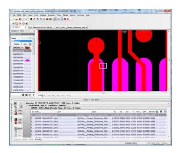
**Solder Mask - Drill Annular Ring** checks include Plated Through Drill to Mask, Unplated Through Drill to Mask, Via Drill to Mask, Laser Via Drill to Mask.
