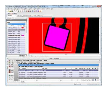
**Solder Mask - Missing Mask** checks include Missing Mask for SMD, Missing Mask for Undrilled Pad, Missing Mask for Unplated Through Drill, Missing Mask for Plated Through Drill, Missing Mask for Via, Missing Mask for Laser Via, and Missing Mask for Testpoint.
