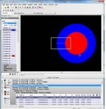
**Negative Plane - Annular Ring** checks include Pad to Drill, Via to Drill, Laser Via to Drill, Blind Via to Drill, Buried Via to Drill, and Pad to Unplated Drill.
