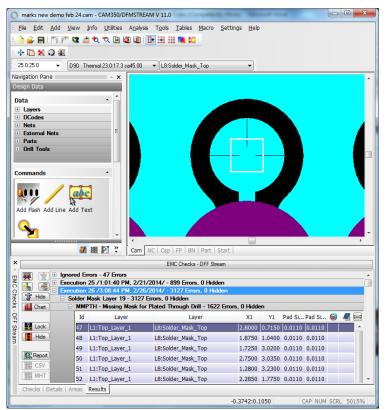
Solder Mask - Extra Mask checks include Missing Copper, and Missing Pad.
